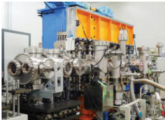
Figure 1: Photograph of the TPS CPMU with an in-situ field measurement system.
