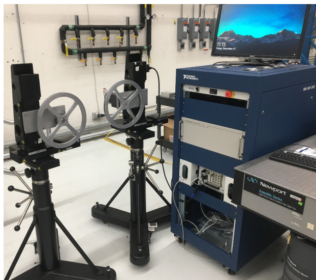
Figure 5: Measurement assemblies including the alignment stands, 3-axis stage assembly, spools, and motors for the Hall sensor. Also pictured is the control rack.
