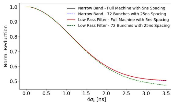
Figure 1: The normalised BPM readout as a function of bunch length for different types of filters and beam parameters. The bunch length at 26 GeV is  $4\sigma_t \approx 2.9$  ns and at 270 GeV it is  $4\sigma_t \approx 1.4$  ns.
