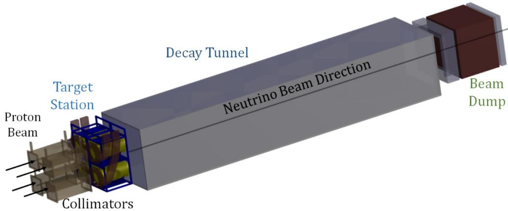
Figure 1: Schematic view of the target/horn station, the tunnel and the beam dump.
