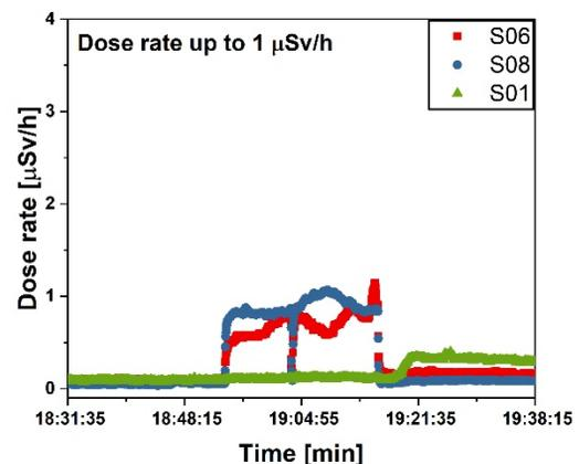
Figure 3: Dose rates during injection after chopper optimization.
