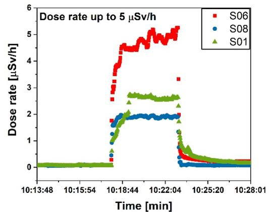
Figure 2: Radiation levels during injection before chopper start-up monitored by 3 RMS.
