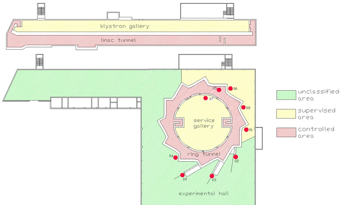
Figure 1: Layout of the Solaris facility.
