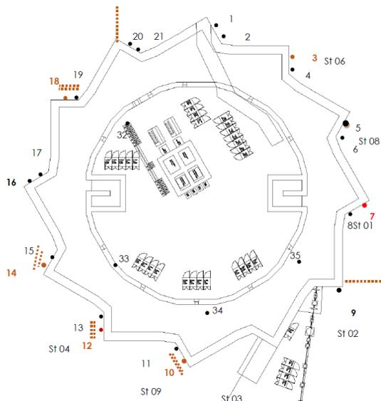
Figure 4: Assessment of radiation levels at higher currents ( $I=350 \text{ mA}$ ). Orange dotted lines indicates places where radiation levels are too high.
