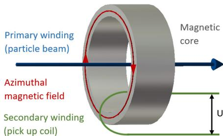
Figure 1: Basic operation principle of AC current clamps.
