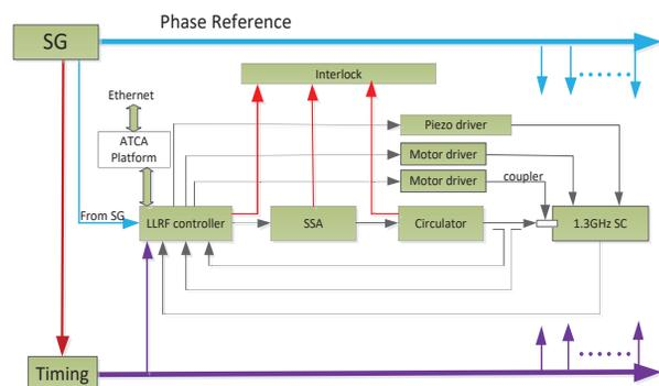
Figure 2: RF station architecture.
