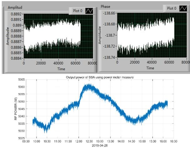
Figure 6: RF stability test result (Up: amplitude and phase stability, Down: power stability).
