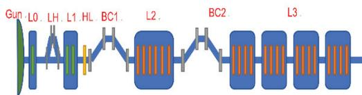
Figure 1: Sketch of SC LINAC for SHINE.
