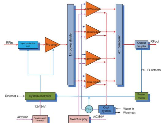
Figure 4: Block diagram of SSA.
