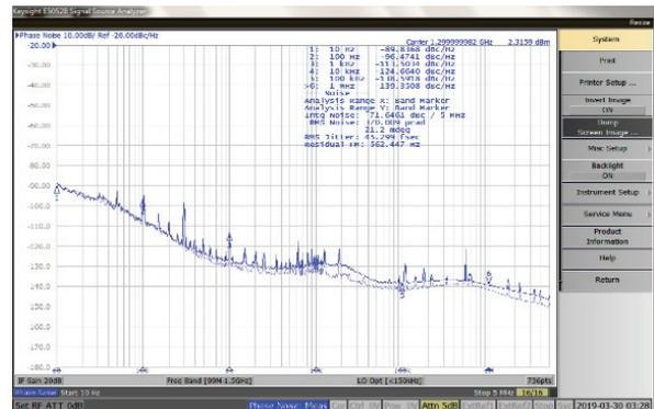
Figure 5: phase noise of SSA output signal and signal generator output signal (thick: SSA output signal, light: signal generator output signal).
