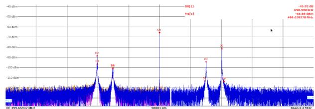
Figure 5: Sum signal of both horizontal and vertical tune frequencies.
