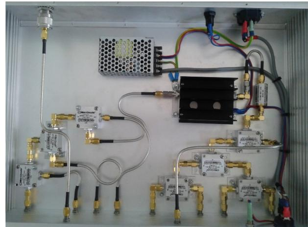
Figure 2: Inside of the MO divider.
