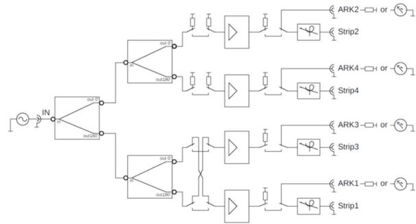
Figure 4: Schematic of the receiving network.
