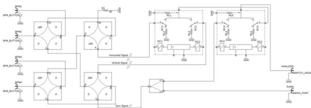
Figure 3: Schematic of the stripline feeding network.
